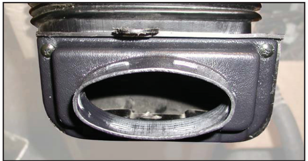
Photo 11 - Install Defrost Duct Adapter
