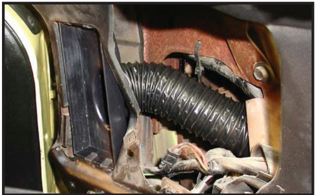
Photo 12 - Drivers Side Duct Adapter
