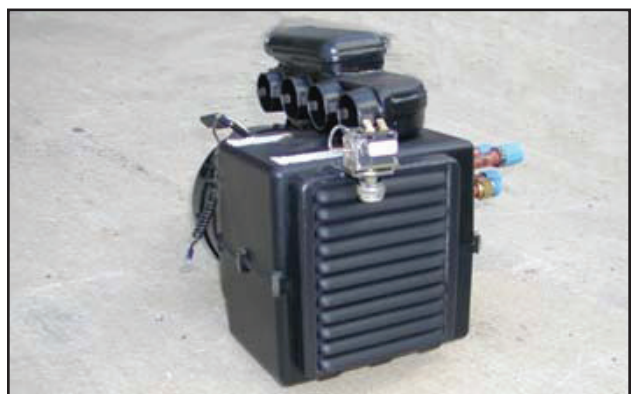
Photo 6 - Install Inlet Grill & Thermostat
