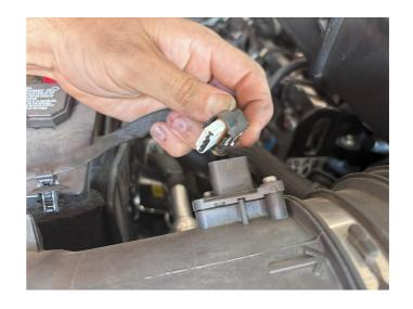
Remove the ribbed push-in clip on the wiring harness from the stock intake lid.
