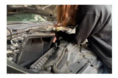
Carefully remove the stock intake filter.
