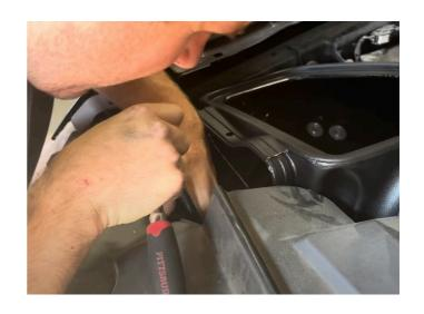
Position the Air Box so that the hole in Air Box is in line and matched with the threaded hole in the fender frame and the holes in the Shoulder Bushings are also in line and matched with the threaded holes in Air Box Bracket. Rotate the Air Box Bracket as required.
